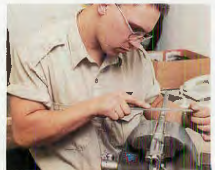
Gunsite custom-shop gunsmith file-finishes the integral barrel scope mounts on the barreled action of a soon-to-be Scout. Photo: courtesy Chris Mayer
